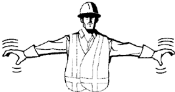
Slack the mainline, easy. Both hands extended at sides, hands fluttering.
