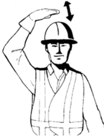
RAISE SKYLINE/GUYLINE Move hand up from top of head several times
