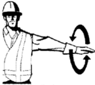
Ahead on haulback, normal speed. One arm extended, rotating.
