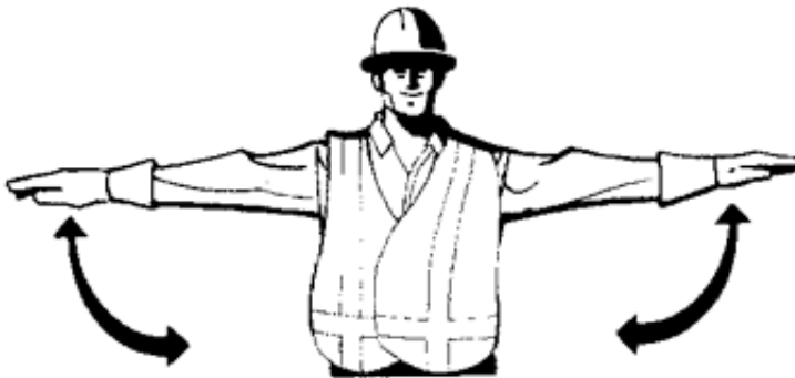
Stop any moving line and hold.
