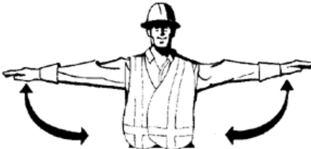
Stop any moving line and hold.
