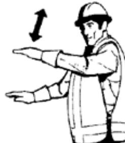
Slack the strawline. Pat back of hand with other hand.
