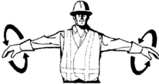
Haulback ahead, slow. Both arms extended, rotating.
