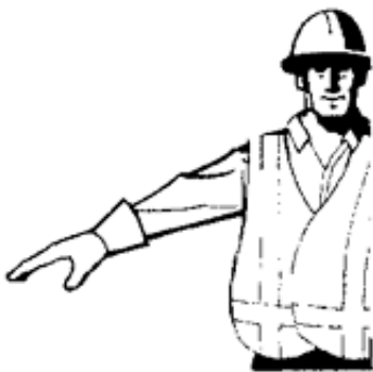
To stop tractor – hold one hand out with palm down.
