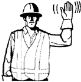
Mainline ahead, fast. One arm raised, hand 'fluttering'.
